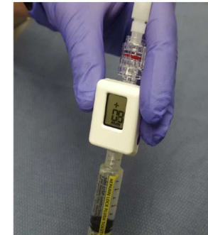
Figure 1. Compact pocket-sized battery-operated manometer.
